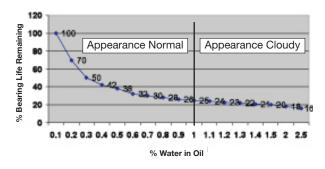
Maintaining minimum water levels is a must. The most common methods of continuous water removal are centrifugal purification for large amounts of water and vacuum dehydration (polishing) for concentrations under 400 ppm.
